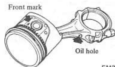
Fig. EM-82 Assembling piston and connecting rod
