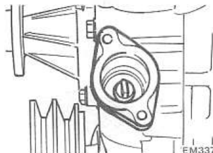
EM337 Fig. EM-103 Setting distributor drive spindle
