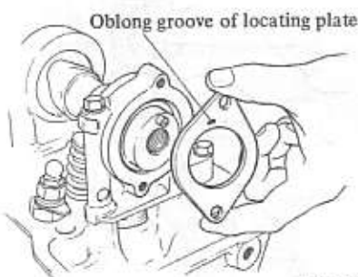
Fig. EM-77 Installing camshaft locating plate
