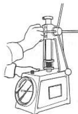
Fig. EM-34 Measuring spring tension
