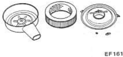
Fig. EF-2 Air cleaner for single carburetor
