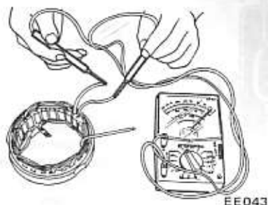
Fig. EE-51 Testing stator for conduction
