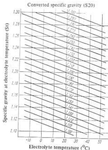
Fig. EE-6 Changes of specific gravity in response to electrolyte temperature change (°C)
